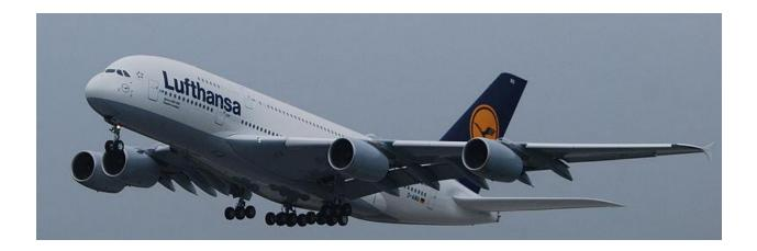
**The Airbus A380** is a double-deck, wide-body, four-engine jet airliner manufactured by Airbus. **It is the world's largest passenger airliner**; many airports have upgraded their facilities to accommodate it because of its size. Initially named Airbus A3XX, Airbus designed the aircraft to challenge Boeing's monopoly in the large-aircraft market; the A380 made its first flight on 27 April 2005 and entered commercial service in October 2007 with Singapore Airlines.
